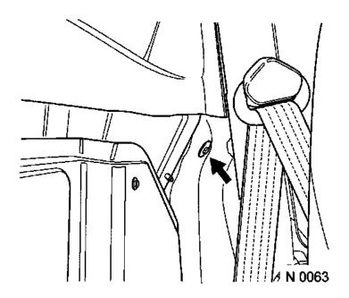
**37.** Release rear header panel from roll bar, then tilt forward
